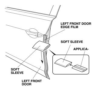
6. Slowly remove the protective film from the left front door edge film.
