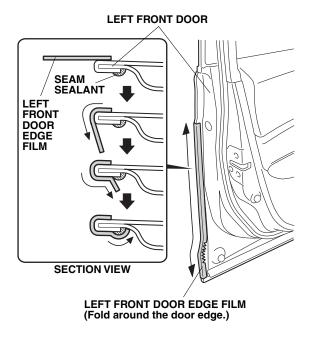
Using a shop towel, wipe the excess 3M protective tape application solution from the left front door edge film. Allow the left front door edge film to dry thoroughly.
