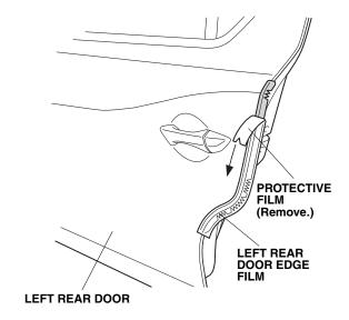
14. Starting from the center and working outward, use your fingers to fold the left rear door edge film around the edge of the left rear door. Move your fingers in one direction. Attach the film over the seam sealant. Do not trim or damage the seam sealant.
